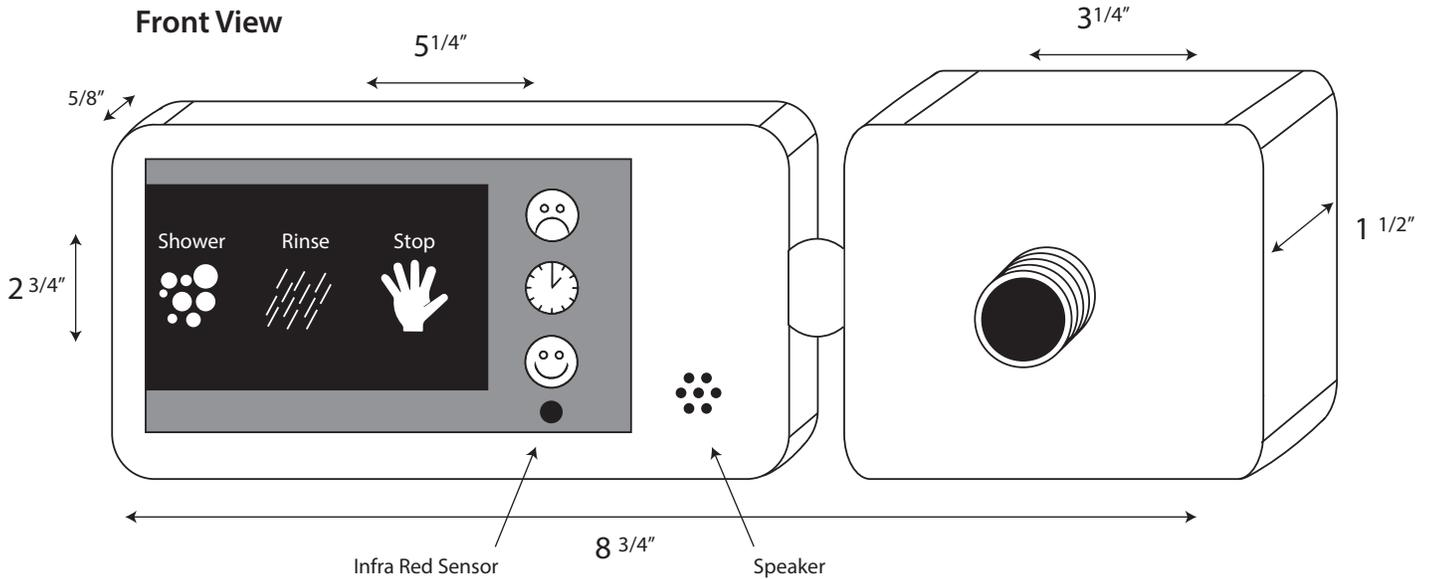
**Infra Red Sensor:** Enables programming via remote control.
